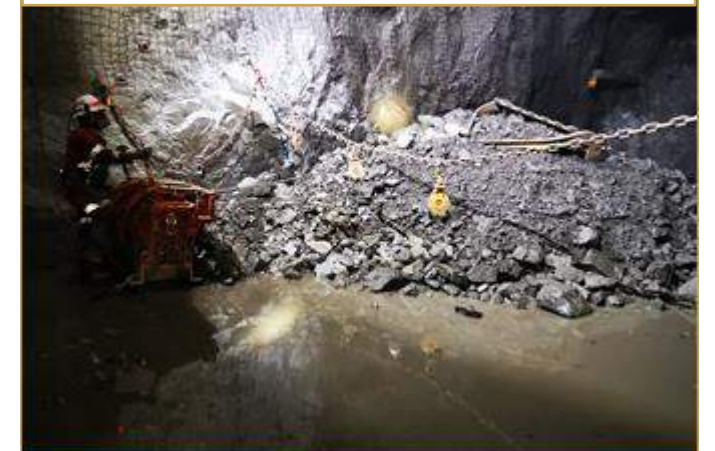
Mucking out a stope with a slusher
