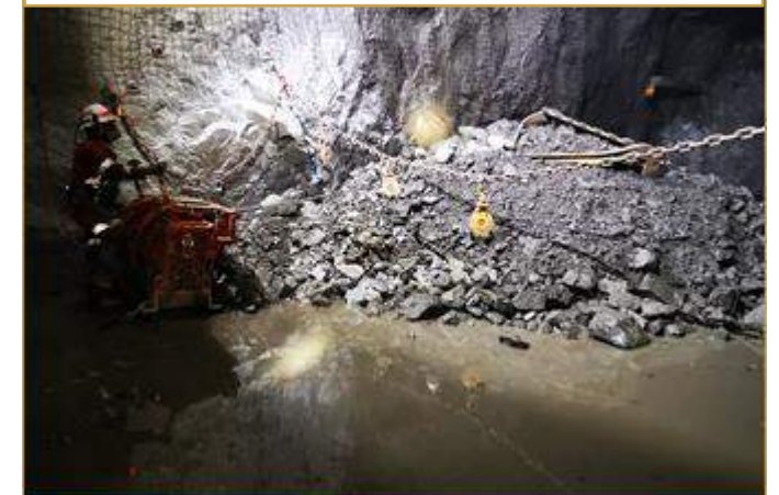
Mucking out a stope with a slusher
