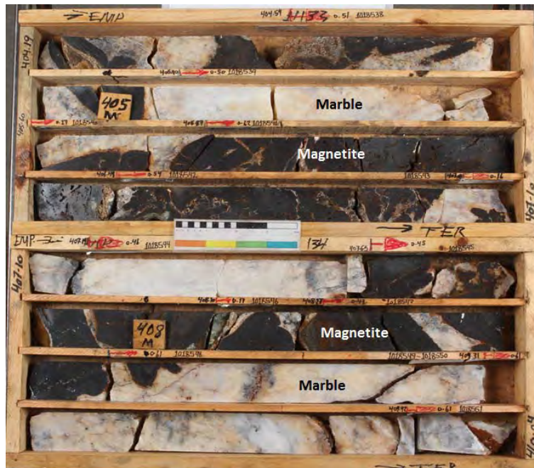
Figure 7-17: Example of Massive Magnetite Bands in White Marble from Drill Hole ML-11A (404.19 m to 410.04 m)
