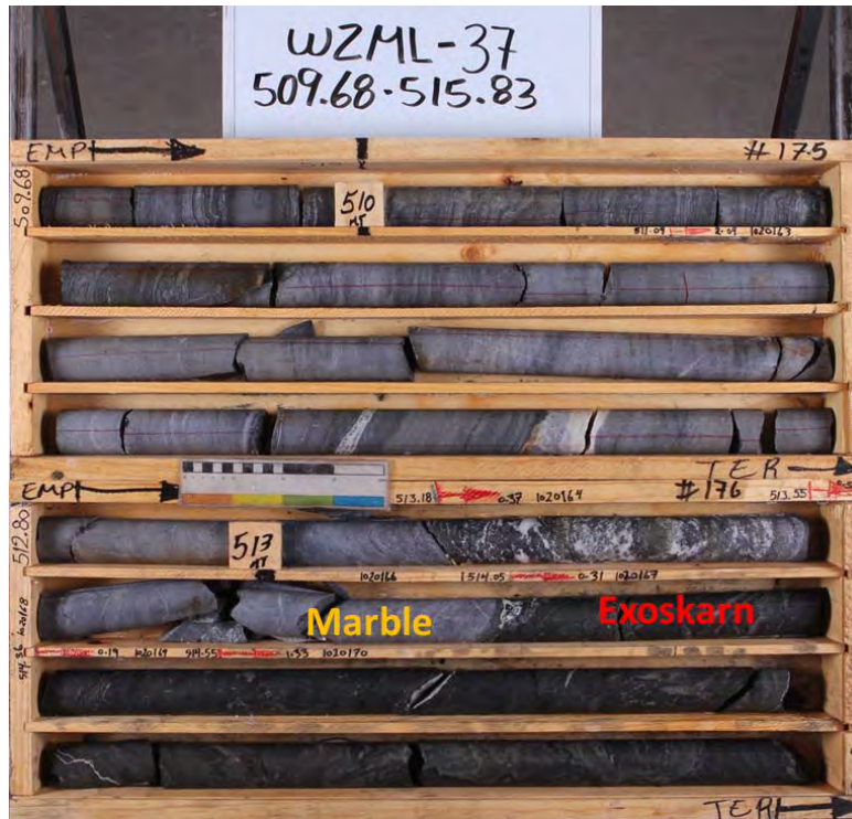
Figure 7-13: Uncut Drill Core from Hole WZML-37 Showing Sharp Marble-Exoskarn Contact at 514.05 m
