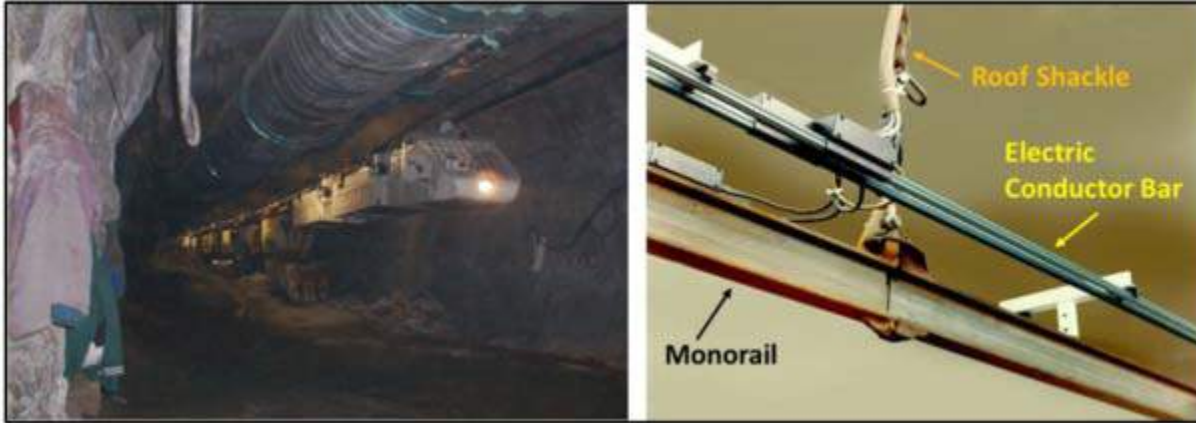
Figure 24-46: Transportation Backbone – Back-Mounted Monorail System (Source SMT Scharf AG)
