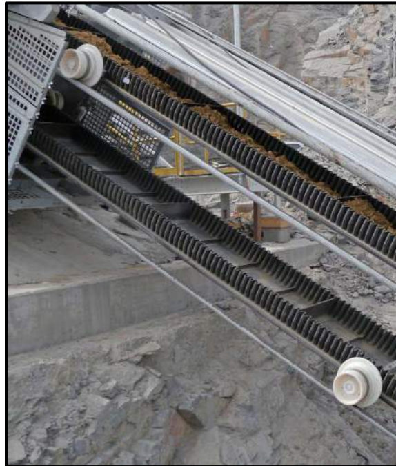
Figure 24-57: El Limon RopeCon - a Suspended Conveyor System at Torex's ELG Mine Complex
